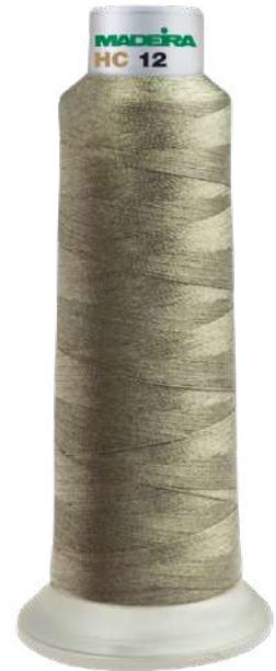
The conductive thread used by Light Stitches is a medium weight and comes on a bobbin of approximately 6M or 150M reel. The thread is much stronger than domestic poly/cotton thread, and somewhat thicker. If using on a machine you may wish to try a larger needle to help with threading up and less chance of fraying by being caught on the point of the needle.
