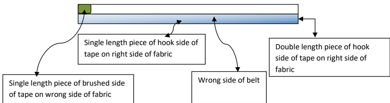
3. The circuitry for the diagonal strap is exactly as per the diagram up above. Sew your circuit into one piece of material with the battery cover at one end. Remember to attach the extra pieces of the brushed side of the hook and loop tape to enable you to fasten the diagonal strap to your waistband.
