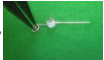
4. Loop the thread through the material and light legs and back through the material. This produces a loop of a smart thread, the needle can then be placed through the loop and pulled tight to produce a knot. Attach two knots, making sure knots are pulled very tight.
