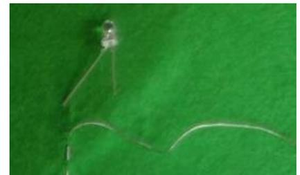
3. Make sure the positive leg (longest leg) of the light is on the left-hand side. Use pliers or scissors to bend each leg round into a loop. Repeat the process for the second light. Making sure the positive leg (longest leg) of the light is on the left-hand side. Finish with a knot.
