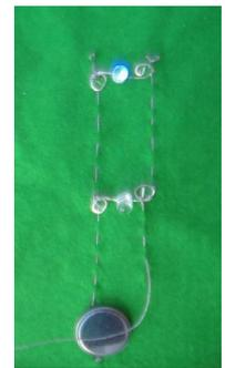
9. If lights do not come on, check lights are attached correctly. (long leg on the left side) Place battery centrally within adhesive part of felt pad, place positive side up.
