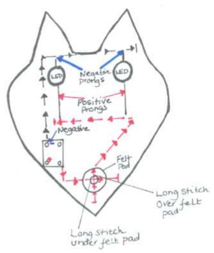
Key = Positive conductive thread statching = Negative conductive thread statching
