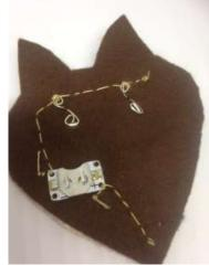
5. Knot conductive thread to the positive hole on the battery holder.
