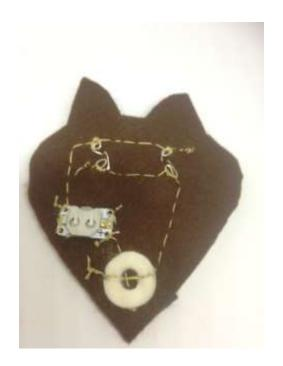
**6.** Stick the soft switch in place over the conductive thread. Sew the conductive thread to lay over the top of the Soft Switch and then running stitch to the positive legs of the LEDs. Sew each LED leg as before finishing with a knot .
