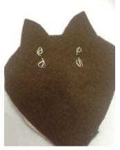
Use the pliers to bend each LED leg round into a loop.
